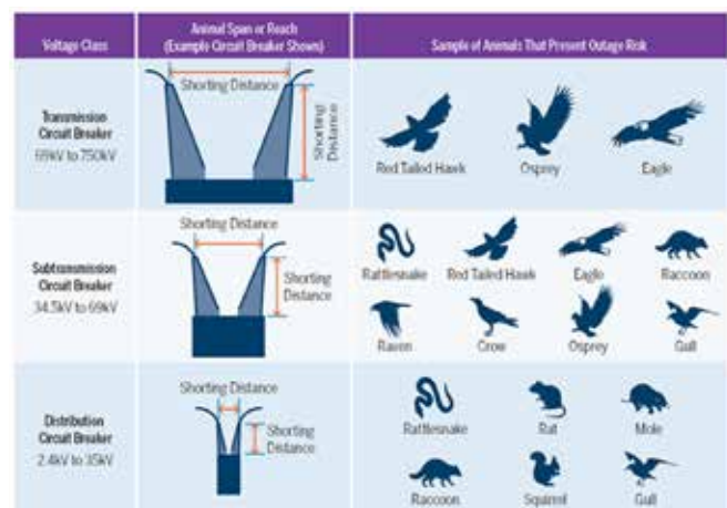
Figure 3: Spacing of Insulators Indicating Shorting Distance. Listing a Sample of Animals That Commonly Bridge the Shorting Distance (not to scale).
